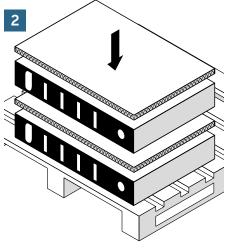
Stack rail free servers onto the pallet with a layer of bubble wrap or cardboard between each layer.
