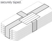
The secure stack of trays needs to be placed into an anti-static bag and wrapped tightly. Each stack should be labelled with the
